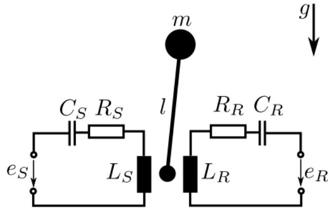
Simulation and control by linear approximations in time, mid-point quadrature for the Lagrangian and forward-rectangle quadrature for the virtual work.
