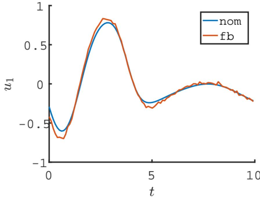
control input (rotor circuit voltage): nominal and feedback-controlled in presence of disturbances
