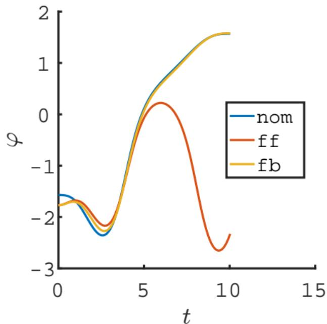
trajectories (pendulum angle): nominal, feed-forward controlled and feedback-controlled in presence of disturbances
